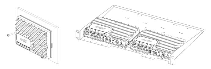
The Aprisa SRi has an earth connection point on the top left and the top right of the enclosure. Use the supplied M4 screws to earth the enclosure to a protection earth.
